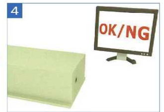
4 Make an OK / NG judgment by image processing while displaying a development image of the inner surface of the cylinder.
